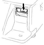
**NOTE:** After replacing the media, press the feed key to confirm that the media is issued correctly. \*Use of other model's label cassette in the SL-9000 may cause a label skew.
